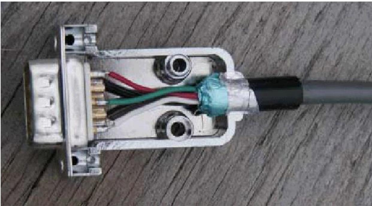
This completes the construction of your transceiver cable assembly. Now it needs to be connected.
