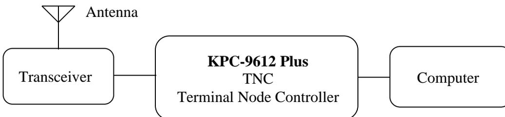
The three parts of a packet radio station work together as follows:
